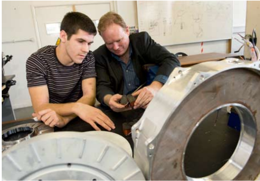
Valentine Ganin, University of Oxford (left) and Prof Malcolm McCulloch, head of Oxford's Electronic Power Group (right). In the foreground is the casing and outer wall of the stator and in the background pole pieces from the stator of the motor
